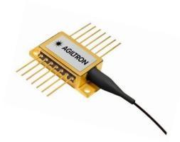
The 1490nm series laser diodes are fabricated in a hermetically sealed 14-pin butterfly package. The laser diodes contain a monitor photodiode, thermoelectric cooler (TEC), and a thermistor to secure high-quality laser performance. Our laser products are Telcordia GR-468 qualified and in compliance with RoHS Directives.
